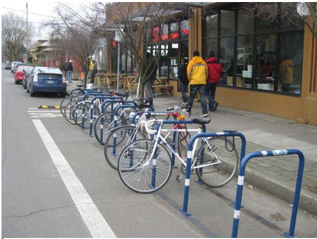
Bike corrals use one vehicle parking space for high-capacity bike parking.
